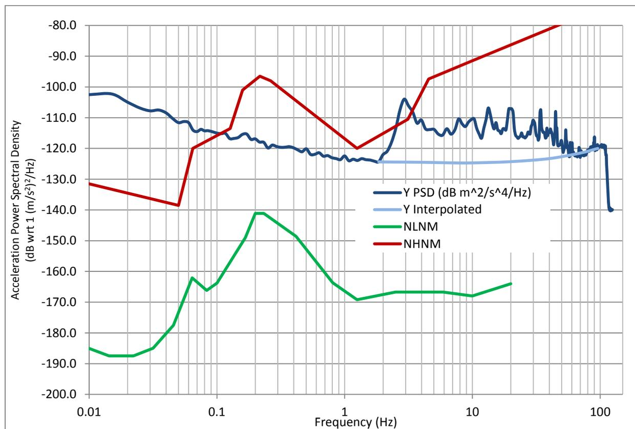
Figure 4 - PSD Self-Noise Showing an Interpolated Y channel Below the Site Noise in the 2-90 Hz Band
