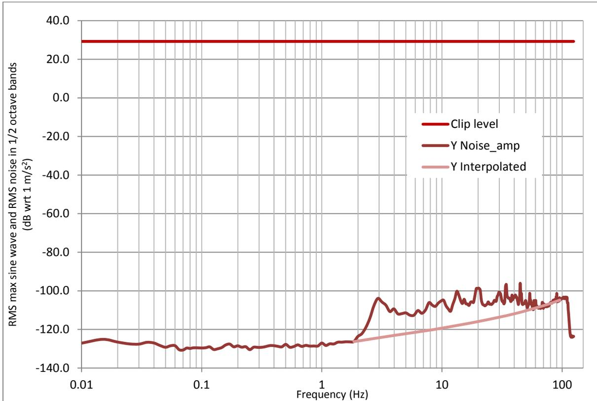
Figure 5 - Comparing RMS Clip Sine Wave to RMS Noise in 1/2 Octave Bands using Interpolated Y Data
