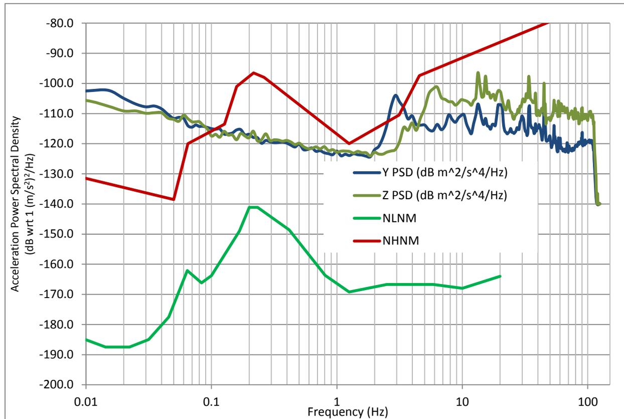
Figure 1- Power Spectral Density of TitanSMA Output Signals with New Low and High Noise Models for Reference
