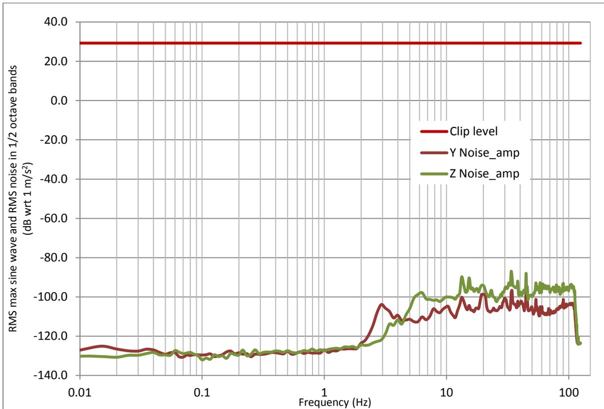
Figure 2 - Comparing RMS Clip Sine Wave to RMS Noise in 1/2 Octave Bands
