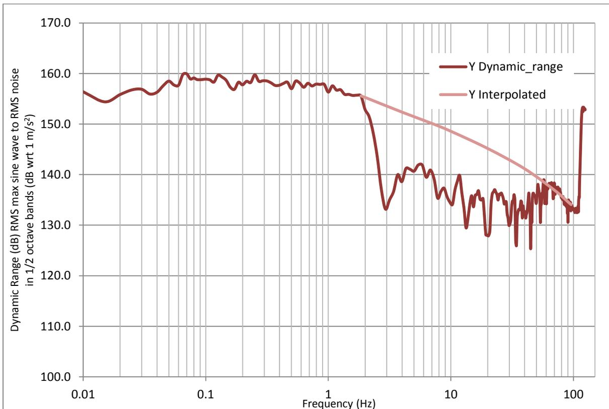
Figure 6 - Dynamic Range Plot using Interpolated Y Data
